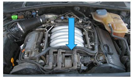
Direct or DIS Ignition will be rectangular with the plug wires arranged in a straight line. The type shown here is a "shared" system. Each coil fires a **pair** of plugs.
